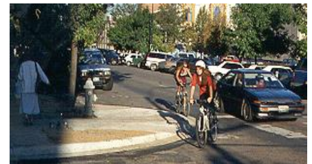
Horizontal —Bulb-out at an intersection
