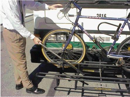
**Step 5:** Pull out and up on the support arm and hook the arm securely over the top of your front wheel. A spring pulls the arm back and holds the bike securely in place.
