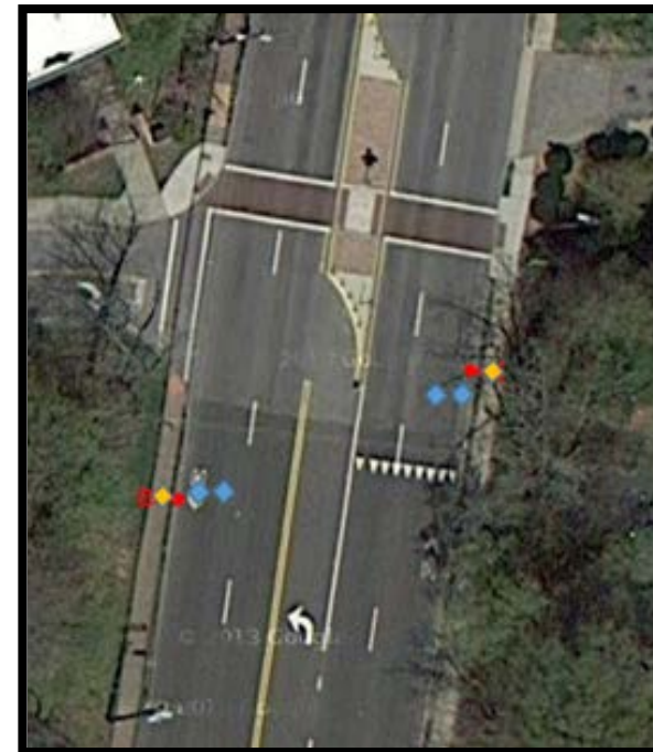
Figure 2. Site diagram showing bicycle and pedestrian count equipment placement
