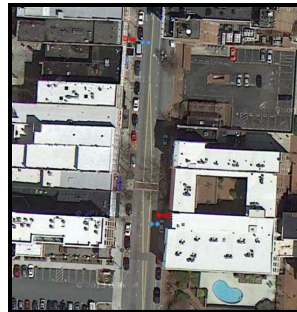
Figure 2. Site diagram showing bicycle and pedestrian count equipment placement
